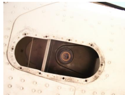
Figure 6: Bottom View of Aircraft Camera Port and Sensor Lens
